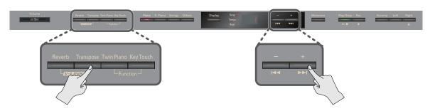
1. While holding down one of the blinking buttons, press the [-] or [+] button to select the setting that you want to edit.
